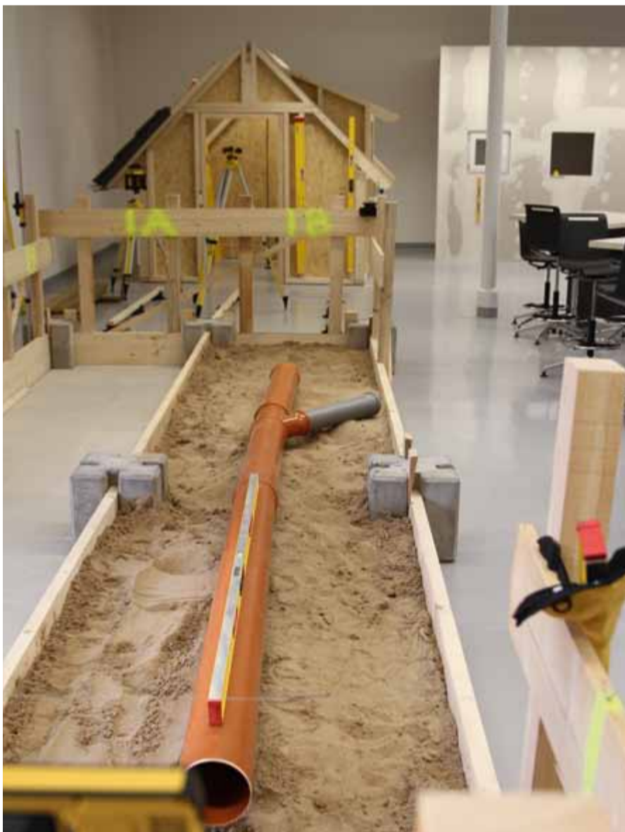
The “sandpit” was designed to demonstrate measuring tasks in underground engineering (e. g. transferring axes, marking walls or creating slopes). Typical carpentry jobs can be demonstrated on and in the timber house: creating right angles, measuring angles and inner dimensions.
